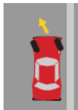
Uphill with curb
